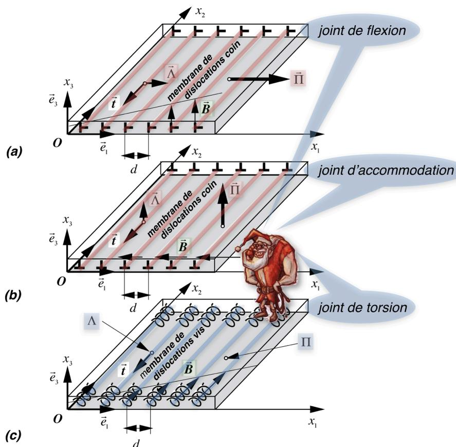
**Figure 2.18** - Membranes de dislocations de type coin:
