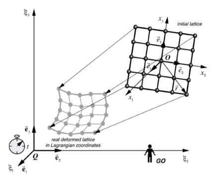
**Figure 2.4** - the displacement field  $\vec{u}_{i}(\vec{r},t)$  in lagrangian coordinates
