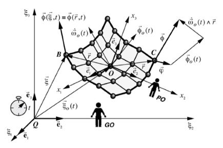
Figure 2.3 - projection of velocity field  $\vec{\phi}$  in the macroscopic local frame
