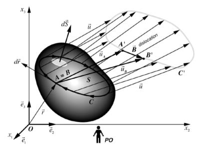
**Figure 3.5** - Interpretation of the condition of compatibility  $\overrightarrow{\text{rot }} \vec{\beta}_i = 0$
