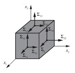
**Figure 6.1** - physical interpretation of the components of the stress tensor  $\tilde{\Sigma}_i$
