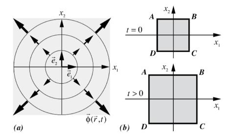
Figure 1.12 - elongations with volume expansion and no shear
