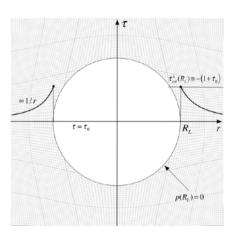
**Figure 22.8b** - The field of expansion of the same macroscopic vacancy with 10'000 sites of lattice when  $\tau_{_0} < -(1 + \tau^{^{external}}(R_{_L}))$ , represented on the same scale as figure 22.8a
