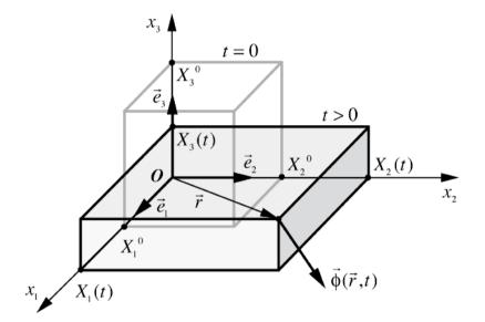
Figure 1.11 - elongations along the axis of coordinates
