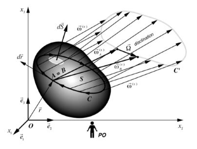
**Figure 3.7** - interpretation of the condition of compatibility rot  $\vec{\chi}_i = 0$
