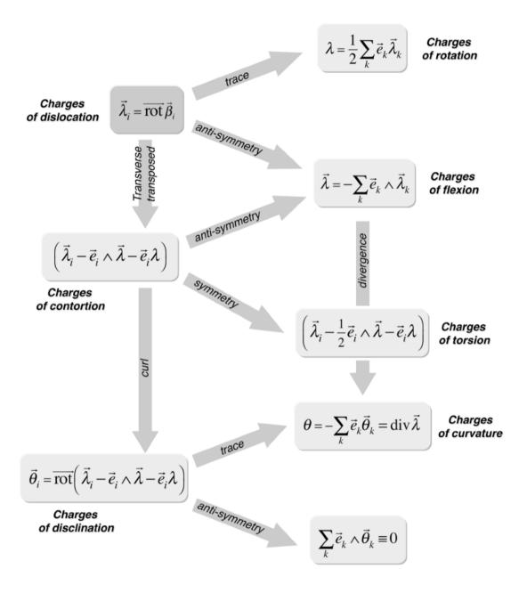
Figure 8.11 - Complete decomposition of the tensorial charges
