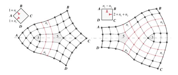
**Figure 9.23 -** doublets  $C1 - \overline{C1}$  of wedge disclinations in a cubic lattice
