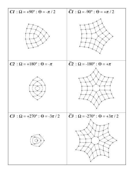
Figure 9.20 - families of quantized wedge disclinations in a quadratic plane arrangement
