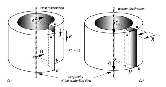
Figure 8.7 - creation of the twist (a) and wedge (b) disclinations by cutting and welding back
