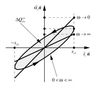
Figure 7.7 - Hysteresis cycle in presence of viscous friction
