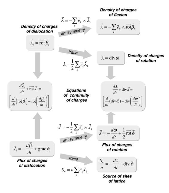
Figure 8.6 - decompositions of the densities and flows of charges and equations of continuity
