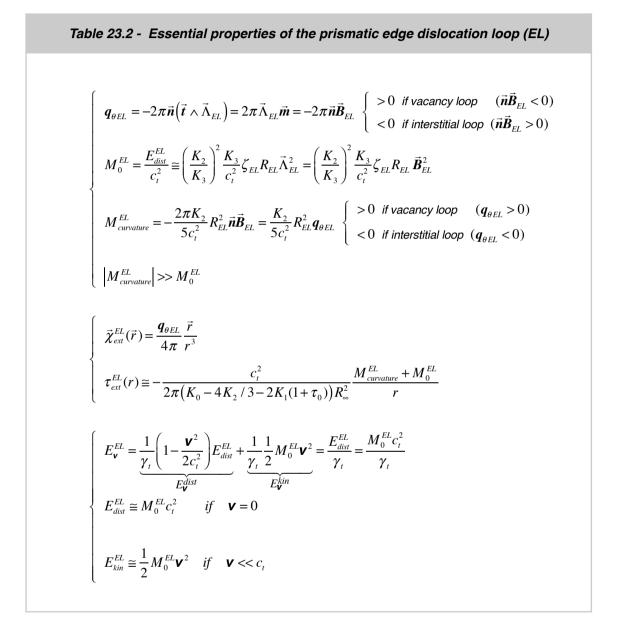
Also, the equivalent gravitational mass of curvature  $M_{curvature}^{EL}$  is not only much larger than the inertial mass  $M_0^{EL}$ , but it can even be negative in the case where the edge loops are interstitials. This is a striking result as it corresponds to the existence of a possible negative gravitational field, and is a new result compared to the General Relativity of Einstein. The possible consequences of this striking result will be explored in more detail in the rest of the book.
