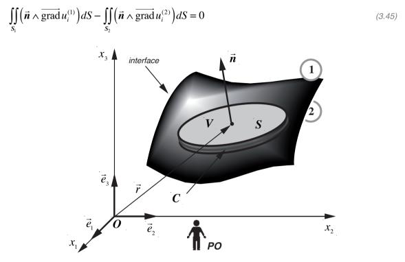
Figure 3.9 - compatible pass-through conditions between 2 solid medium
