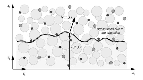
Figure 12.9 - The stress fields due to obstacles represented in the slip plane
