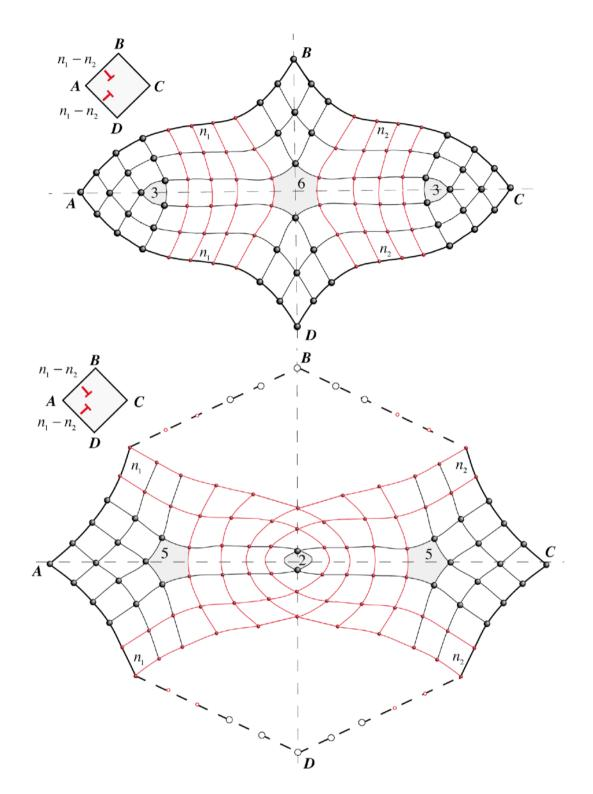
**Figure 9.26 -** triplets  $C1 - \overline{C2} - C1$  and  $\overline{C1} - C2 - \overline{C1}$  of wedge disclinations in a cubic lattice
