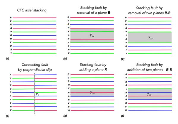
**Figure 31.16 -** The three types of faults between axial dense planes, by perpendicular slip (d), by removal (b,c) or addition (e,f) of one or two dense planes, with respectively fault energies  $\gamma_0$ ,  $\gamma_{1a}$  and  $\gamma_{1b}$
