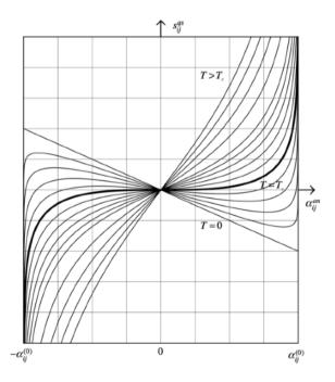
Figure 7.14 - the anelastic stress-strain  $s_{ij}^{\scriptscriptstyle qs} - lpha_{ij}^{\scriptscriptstyle an}$  diagram
