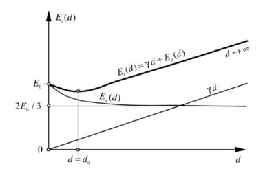
Figure 9.10 - The energy of two partial dislocations as a function of the distance that separates them
