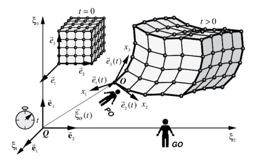
**Figure 2.2** - the solid lattice around the neighborhood of point **0** with local frame  $Ox_1x_2x_3$
