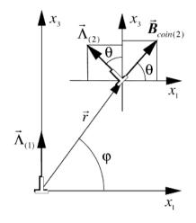
Figure 12.3 - interaction between two parallel edge dislocations along  $Ox_2$ with charges  $\vec{\Lambda}_{(1)}$  and  $\vec{\Lambda}_{(2)}$
