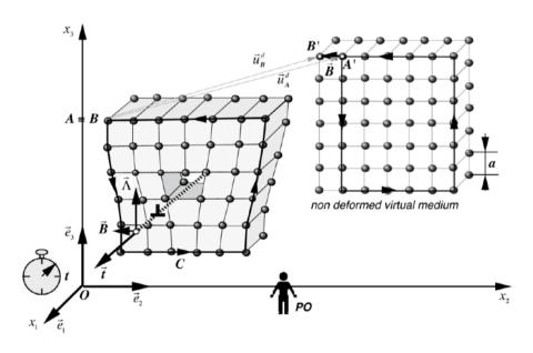
Figure 9.3 - edge dislocation is quantified in a cubic lattice
