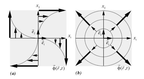
Figure 1.17 - examples of non-uniform distortions
