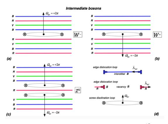
**Figure 31.5** - Intermediate bosons formed by screw disclination loops of angle  $\pm 2\pi$ which do not need edge dislocation loops to ensure the continuity of succession of **R**,**B**,**V** planes
