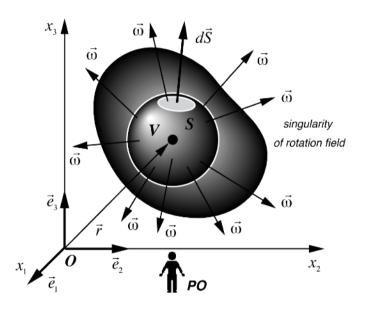
**Figure 3.6** - interpretation of the condition of compatibility  $\operatorname{div} \vec{\omega} = 0$
