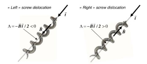
Figure 9.4 - screw dislocation, left and right respectively
