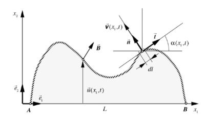
**Figure 12.7** - definition of displacement  $\vec{u}(x, t)$  of a dislocation in its slip plane
