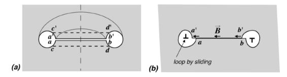
Figure 8.4 - cut of a torus and the median plane to form loops (a) and creation of a dislocation loop by sliding of the jaws (b)
