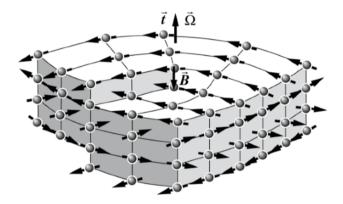
**Figure 9.34** - dispiration of +90° introduced in the axial medium of figure 9.32 (b) showing the need to add a translation vector  $\vec{B}$  to insure axial continuity
