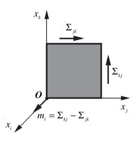
Figure 9.3 - physical interpretation of the components of the torque vector or torsor of moment  $\vec{m}$
