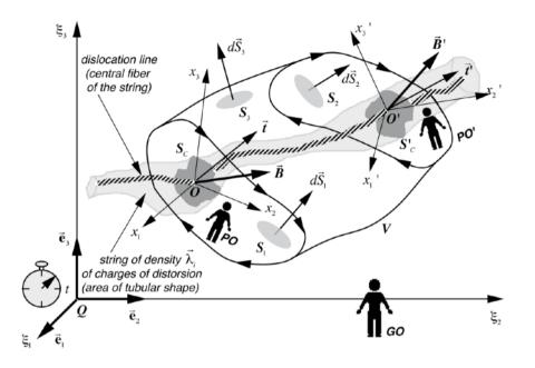
**Figure 9.1 -** string (domain of tubular shape) of density  $\vec{\lambda}_i$  of charges of distortion and the dislocation line (central fiber of the string)
