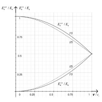
**Figure 20.5** - Fractions of total energy under a potential and kinetic form as a function of  $\mathbf{v} / c_i$ , in the case of a screw or edge dislocation (1) or a spherical charge of rotation (2)
