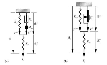
*Figure 7.8* - rheological models (*a*) with viscous friction and inertial mass (*b*) with a dry friction pad
