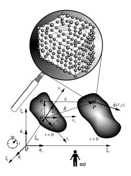
Figure 1.1 - spatiotemporal evolution of a medium in the absolute frame
