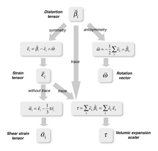
Figure 1.8 - Decomposition of the eulerian tensor of distortions
