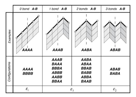
Figure 7.16 - the 16 possible configurations of the 4 successive atomic planes
