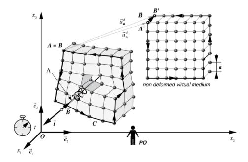
Figure 9.2 - screw dislocation is quantified in a cubic lattice
