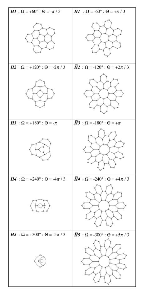
Figure 9.21 - families of quantized wedge disclinations in a hexagonal plane arrangement
