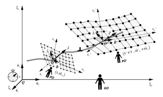
Figure 9.12 - effects of a spatial variation of the volume expansion on a lattice dislocation
