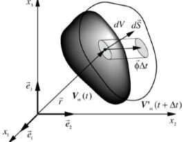
Figure E.4 - derivative of an integral on a mobile volume
