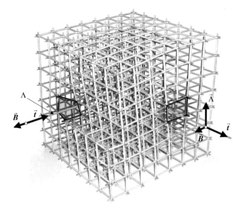
Figure 9.6 - dislocation changing from a screw type to an edge type in a cubic lattice
