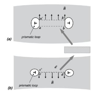
Figure 8.5 - creation of prismatic loops of dislocation by addition (a) or subtraction (b) of thin disk of material
