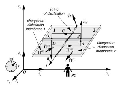
Figure 9.16 - string of disclination at the frontier of two membranes of dislocations
