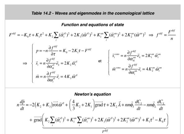
Propagation of transversal waves coupled to longitudinal wavelets
