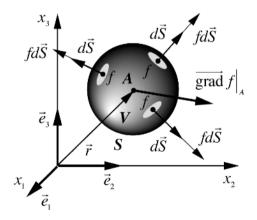
Figure E.1 - gradient operator
