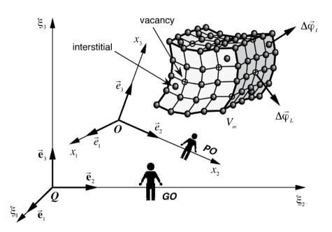
Figure 5.3 - flux of vacancies and interstitials across the surface of a chunk of lattice
