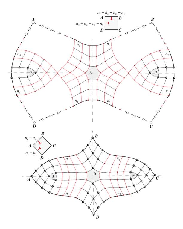
Figure 9.25 - triplets  $C1 - \overline{C}2 - C1$  of wedge disclinations in a cubic lattice
