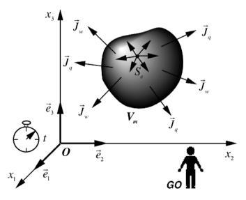
**Figure 4.1** - mass flux  $\vec{J}_m$ , work flux  $\vec{J}_w$ , heat flux  $\vec{J}_q$ , source of mass  $S_m$  and source of entropy density  $S_e$  on a given mobile volume  $V_m$  of medium
