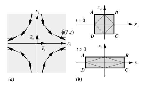
Figure 1.13 - elongations with null volume expansion (constant volume)
