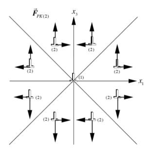
**Figure 12.4** - components of the force of Peach and Koehler due to the interaction between two edge dislocations parallel to axis  $Ox_2$  and with charges  $\vec{\Lambda}_{(1)}$  and  $\vec{\Lambda}_{(2)}$  along the axis  $Ox_3$
