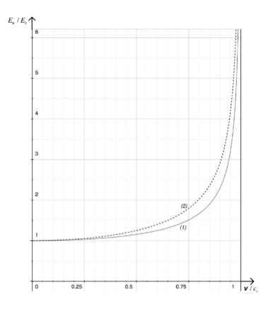
**Figure 20.4** - The total energy compared to the rest energy as a function of  $\mathbf{v} / c_r$ , in the case of a screw or edge dislocation (1) or a charge of rotation (2)
