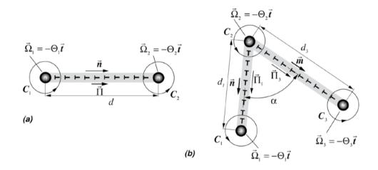
Figure 9.29 - ribbons of virtual dislocations of a doublet (a) and a triplet (b) of wedge disclinations
