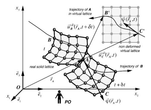
**Figure 2.9** - interpretation of the partial derivative of the local field  $\vec{u}_{E}^{(\delta)}$  with respect to time
