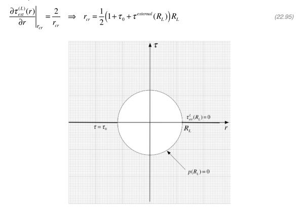
Figure 22.8a - The null field of expansion  $au_{_{ext}}^{^{(L)}}(r)$  of a macroscopic vacancy
