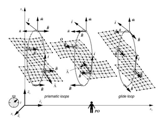
Figure 9.37 - quantification of the dislocation loops on a lattice
