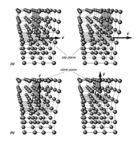
Figure 10.3 - movement of slipping (a) and climbing (b) of an edge dislocation
