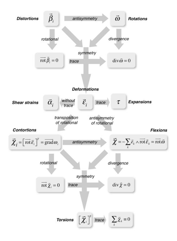
Figure 3.4 - complete description of the distortions and contortions of a compatible solid lattice
