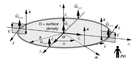
Figure 9.40 - loop of twist disclination with its charged membrane
