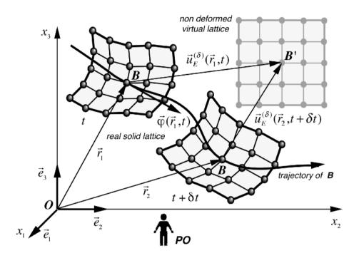
**Figure 2.8** - relation between the local field velocity  $\vec{\phi}$  and the field of local displacement  $\vec{u}_{F}^{(\delta)}$
