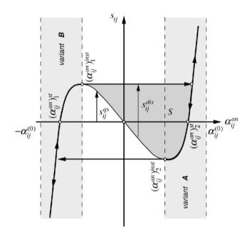
**Figure 7.15** - Hysteresis cycle  $s_{ij} - \alpha_{ij}^{an}$  in the domain of temperature  $T < T_c$
